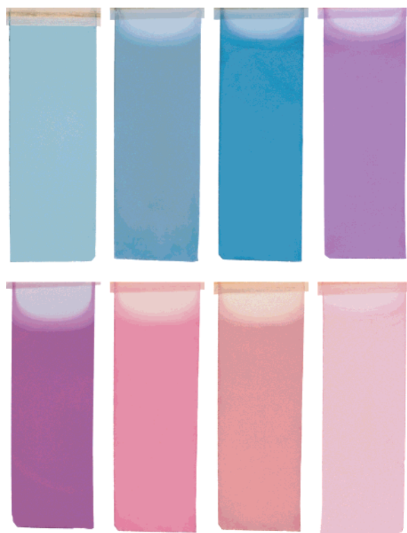
Figure 4. Photographs of dense Au@SiO 2 films with 15-nm-diameter core gold particles and different shell thicknesses. The top left film is a sputter-coated gold film. The next two bluish films are formed from gold sols that have sodium citrate (0.5 nm) and sodium mercaptopropionate (1.0 nm) shells; the other films utilize gold colloids with silica shells having thicknesses 1.5, 2.9, 4.6, 12.2, and 17.5 nm. The shell thickness controls the dipole coupling between particles and hence the color of the film. Reprinted with permission from ref 34. Copyright 2000 The Royal Society of Chemistry.
